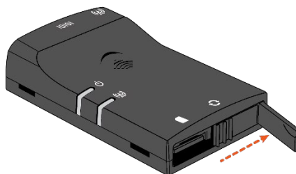
Figure 5 – Revealing the SIM card slot
